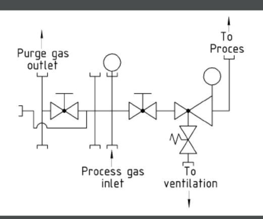
Cylinder station with inlet and outlet gauge, shut-off valve, shut-off valve for process and purge gas. Completely mounted on a wall bracket out of stainless steel.
